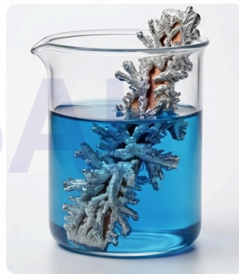
Final: Solution turns blue ( \text{Cu}^{2+} ). Shiny silver deposits.
