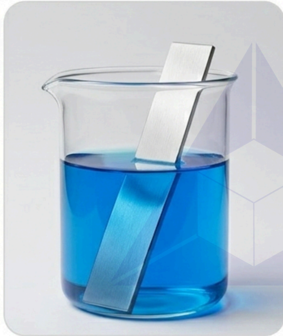
Panel 1 (Left) Initial: Deep blue \text{Cu}^{2+} solution.
